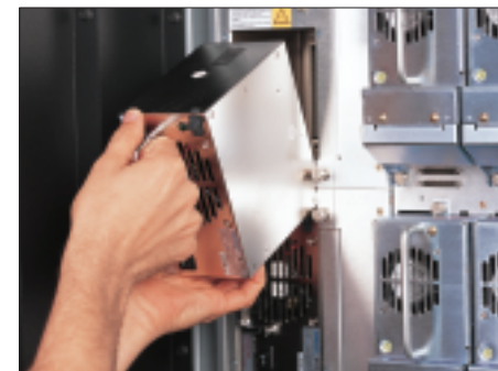
The NEO SERIES features redundant power supplies that can be replaced without interruption.
