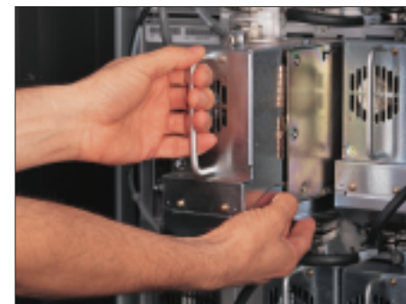
NEO's LiveSwap™ lets you move tape drives without interrupting SCSI bus operations.
