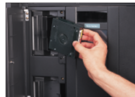
Mailslot design means you can add and remove cartridges easily without disrupting the system.
